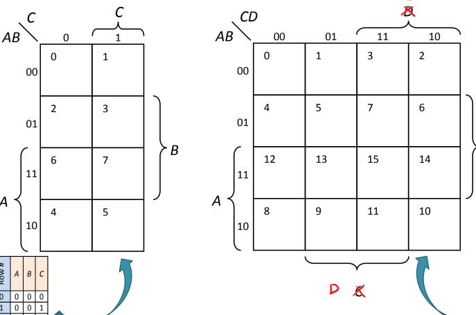
The small number inside each cell is the corresponding row number in the truth table, assuming that the truth table inputs are labeled alphabetically from left to right (e.g. *A*, *B*, *C*) and the rows are numbered in binary counting order.
